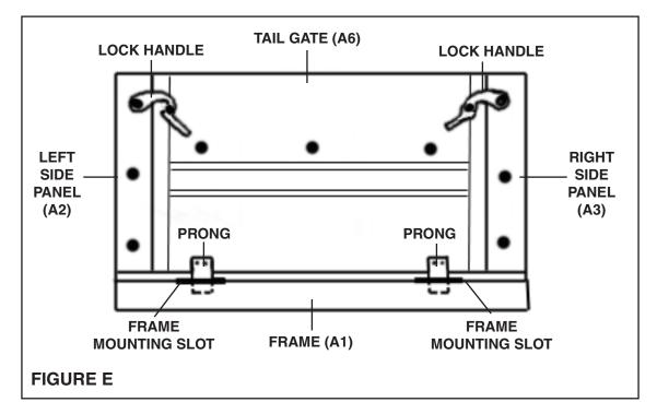
6. Raise the Lock Handles on the rear of the Left Side Panel (A2) and Right Side Panel (A3). Insert the Tail Gate between the Left Side Panel and Right Side Panel. Make sure the two Prongs at the bottom of the Tail Gate are inserted into the two Mounting Slots in the rear of the Frame (A1). Then, lower the Lock Handles to lock the Tail Gate in position. (See Figure E.)
